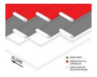
felt ply. Place two rows of fasteners, with the rows spaced approximately 11" (279 mm) apart, and fasteners staggered on approximately 1/8" (457 mm) centers. Use fasteners appropriate to the insulation and deck.
