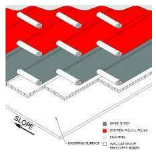
fiber glass base sheet through the insulation into the deck (metal, structural concrete, gypsum, cementitious wood fiber).
