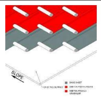
4. Starting at the low point of the roof heat, weld a full width piece of Dibiten Granular or Dibiten FR so that it is firmly and uniformly set. Subsequent sheets are to be applied in the same manner, with 4" (102 mm) side and 6" (152 mm) end laps over the preceding sheets. All laps must be rolled with a 3" (76 mm) rounded edge roller. A 1/8" to 3/8" (3 mm to 10 mm) bleedout of compound shall be visible at the edge of all seams. All laps must be checked for good adhesion.
