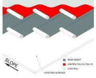
cold adhesive to structural concrete, cementitious wood fiber and pre-cast concrete decks.
