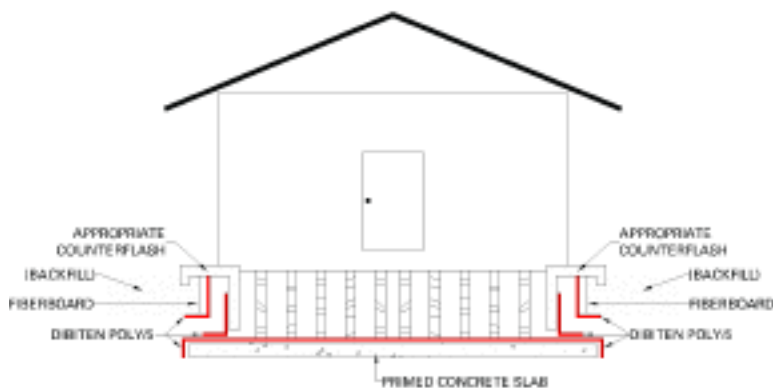
Example Above: Below-Grade Waterproofing (ex: Foundations)
