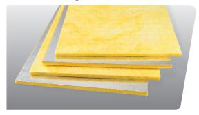
Micro-Aire® LP (Low Pressure) is an FSK-faced fiberglass duct board, designed to be fabricated into ducts for modular housing. Micro-Aire LP offers improved thermal and acoustical control for systems that operate within relatively low air velocities (2,000 fpm).
