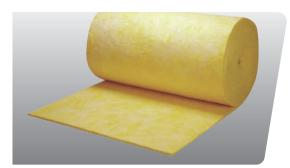
Spiral SG® is a fiberglass insulation designed for double-wall applications. The insulation comes in a variety of thicknesses to help optimize thermal and acoustical performance. It is made from rotaryprocess glass fibers bonded with a thermosetting resin, improving tensile strength and flexibility, and making it resistant to damage during installation
