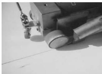
To hot air weld, insert the nozzle fully into the 2" (5.08 cm) weld zone, and raise the back wheel to allow the machine to ride on its two drive wheels. Dial in the desired temperature and speed.
