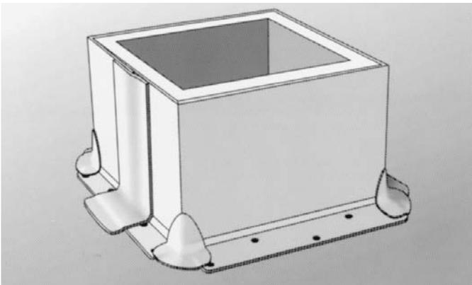
Install JM PVC Universal Corners, welded to the JM PVC-Coated Metal Flashing with a continuous 1" (2.54 cm) minimum heat weld. Care must be taken to leave an unwelded area at the center of the corner to allow for movement.
