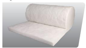
HTB 26 Spin-Glas® is a lightweight, fiberglass blanket insulation designed for industrial applications. HTB 26 Spin-Glas is an excellent choice for applications requiring a low-density blanket. In addition, its high tensile strength provides resistance to damage during installation. This flexible blanket is ideal for heated, irregular surfaces. The insulation is US Coast Guard approved and complies with US Navy and Nuclear Regulatory Commission product standards.
