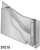
6" (152 mm) 25 gauge steel studs: single layer 5/8" (16 mm) Type X gypsum board each side; one thickness 61/2" (165 mm) JM Formaldehyde-free thermal/acoustical fiber glass batts.
