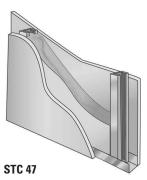
2 1/z" (64 mm) steel studs: single layer 5/s" (16 mm) Type X gypsum board each side; one thickness 2 3/4" (70 mm) JM Formaldehyde-free thermal/acoustical fiber glass batts.
