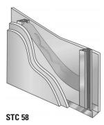
6" (152 mm) 25 gauge steel studs: double layer  $^5/8$ " (16 mm) Type X gypsum board each side; one thickness 6  $^1/2$ " (165 mm) JM Formaldehyde-free thermal/acoustical fiber glass batts.
