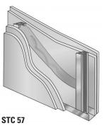
21/2" (64 mm) steel studs: double layer 5/8" (16 mm) Type X gypsum board each side; one thickness 23/4" (70 mm)
