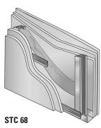
6" (152 mm) 20 gauge steel studs, resilient channels: three layers \(^5/8\)" (16 mm) Type X gypsum board one side, double layer \(^5/8\)" (16 mm) Type X gypsum board other side; one thickness \(^61/2\)" (165 mm) JM Formaldehyde-free thermal/acoustical fiber glass batts.
