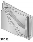
2 ¹/z" (64 mm) steel studs: double layer ¹/z" (13 mm) Type X gypsum board each side; one thickness 2 ³/4" (70 mm) JM Formaldehyde-free thermal/acoustical fiber glass batts.
