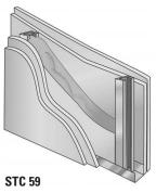
35/s" (92 mm) steel studs: double layer 5/s" (16 mm) Type X gypsum board each side; one thickness 35/s" (92 mm) JM Formaldehyde-free thermal/acoustical fiber glass batts.
