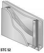
$2^{1/2}$  (64 mm) steel studs: double layer  $^{5}/\!\!/^{\rm s}$  (16 mm) Type X gypsum board one side, single layer other side; one thickness  $2^{3}/\!\!/^{\rm s}$  (70 mm) JM Formaldehyde-free thermal/acoustical fiber glass batts.
