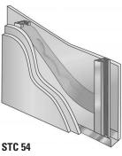
6" (152 mm) 25 gauge steel studs: double layer  $^5/^{\rm s}$  (16 mm) Type X gypsum board one side, single layer other side; one thickness  $6\,^1/^{\rm s}$  (165 mm) JM Formaldehyde-free thermal/acoustical fiber glass batts.
