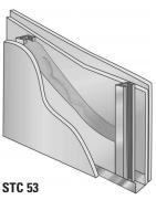
$3^5/8$ " (92 mm) steel studs: double layer 1/2" (13 mm) Type X gypsum board one side, single layer other side; one thickness  $3^5/8$ " (92 mm) JM Formaldehyde-free thermal/acoustical fiber glass batts.
