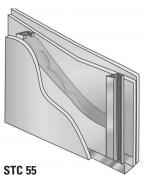
35/s" (92 mm) steel studs: double layer 5/s" (16 mm) Type X gypsum board one side, single layer other side; one thickness 35/s" (92 mm) JM Formaldehyde-free thermal/acoustical fiber glass batts.
