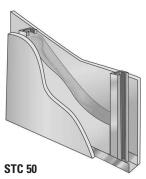
35/s" (92 mm) steel studs: single layer 5/s" (16 mm) Type X gypsum board each side; one thickness 35/s" (92 mm) JM Formaldehyde-free thermal/acoustical fiber glass batts.
