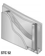
$2^{1/2}$ " (64 mm) steel studs: double layer  $^{1/2}$ " (13 mm) Type X gypsum board one side, single layer other side; one thickness  $2^{3/4}$ " (70 mm) JM Formaldehyde-free thermal/acoustical fiber glass batts.
