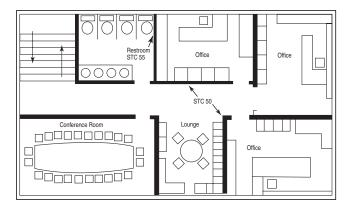
The following examples of different steel stud wall systems demonstrate improved STC values by the inclusion of Johns Manville sound control insulation between metal studs, 24" (610 mm) on center.
