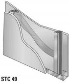
35/s" (92 mm) steel studs: single layer 1/2" (13 mm) Type X gypsum board each side; one thickness 35/s" (92 mm) JM Formaldehyde-free thermal/acoustical fiber glass batts.
