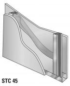
2 1/2" (64 mm) steel studs: single layer 1/2" (13 mm) Type X gypsum board each side; one thickness 2 3/4" (70 mm) JM Formaldehyde-free thermal/acoustical fiber glass batts.
