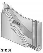
6" (152 mm) 25 gauge steel studs, resilient channels: double layer 5/8" (16 mm) Type X gypsum board one side, single layer other side; one thickness 6 1/2" (165 mm) JM Formaldehyde-free thermal/acoustical fiber glass batts.
