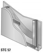
6" (152 mm) 20 gauge steel studs, resilient channels: single layer 5/8" (16 mm) Type X gypsum board each side; one thickness 6 1/2" (165 mm) JM Formaldehyde-free thermal/acoustical fiber glass batts.
