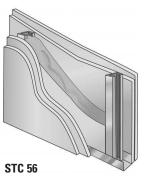
$3\,^5/\!\!\!e^{\rm *}$  (92 mm) steel studs: double layer  $^1/\!\!\!e^{\rm *}$  (13 mm) Type X gypsum board each side; one thickness  $3\,^5/\!\!e^{\rm *}$  (92 mm) JM Formaldehyde-free thermal/acoustical fiber glass batts.
