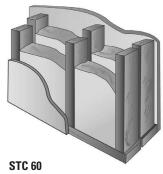
Double 2" x 4" (51 mm x 102 mm) wood studs 24" OC (610 mm): single layer  $^{1}/_{2}$ " (13 mm) Type X gypsum board each side; two thicknesses 35/8" (92 mm) JM Formaldehyde-free thermal/acoustical fiber glass batts.
