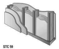
Staggered 2" x 4" (51mm x 102mm) wood studs 24" OC (610 mm): double layer 1/2" (13 mm) Type X gypsum board one side, single layer other side; one thicknesses 3 5/8" (92 mm) JM Formaldehyde-free thermal/acoustical fiber glass batts.
