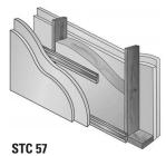
Single 2" x 4" (51 mm x 102 mm) wood studs 24 0C (610 mm), resilient channels: double layer  $^{1}/_{2}$ " (13 mm) Type X gypsum board each side; one thickness  $3\,^{5}/_{8}$ " (92 mm) JM Formaldehydefree thermal/acoustical fiber glass batts.
