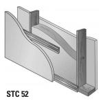
Single 2" x 4" (51 mm x 102 mm) wood studs 24" OC (610 mm), resilient channels: single layer 5/s" (16 mm) Type X gypsum board each side; one thickness 3 5/s" (92 mm)
