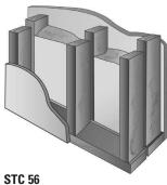
Double 2" x 4" (51 mm x 102 mm) wood studs 16" OC (406 mm): single layer  $^{1}/_{2}$ " (13 mm) Type X gypsum board each side; one thickness 3 5/8" (92 mm) JM Formaldehyde-free thermal/acoustical fiber glass batts.
