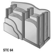
Double 2" x 4" (51 mm x 102 mm) wood studs 16" OC (406 mm): double layer 1/2" (13 mm) Type X gypsum board one side, single layer other side; two thicknesses 3 5/8" (92 mm) JM Formaldehyde-free thermal/acoustical fiber glass batts.
