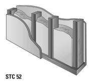
Staggered 2" x 4" (51 mm x 102 mm) wood studs 16" OC (406 mm): single layer 1/2" (13 mm) Type X gypsum board each side; one thickness 3 5/8" (92 mm) JM Formaldehyde-free thermal/acoustical fiber glass batts.
