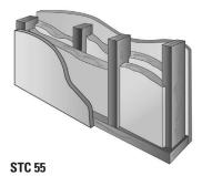
Staggered 2" x 4" (51 mm x 102 mm) wood studs 16" OC (406 mm): single layer 1/2" (13 mm) Type X gypsum board each side; two thicknesses  $3\,^{5}/_{8}$ " (92 mm) JM Formaldehyde-free thermal/acoustical fiber glass batts.
