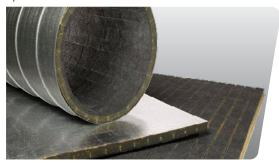
Spiracoustic Plus® is a fiberglass insulation designed to line spiral ducts. It has factory-made, evenly spaced kerfs to allow the material to easily conform to the inside diameter of spiral air ducts. The airstream surface and transverse edges are protected with JM's factory-applied Permacote coating. Spiracoustic Plus can save time and reduce weight when compared to some double-wall systems.
