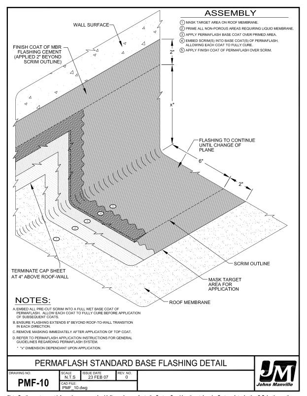
Note: For the most current information on general guidelines, please refer to the System Considerations tab under Systems Introduction & Selection on the JM Roofing Web site. For specifications, flashing details and general installation information please refer to the System Application tab.
