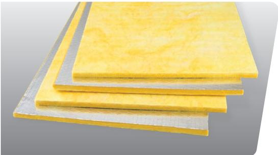
Micro-Aire® LP (Low Pressure) is an FSK-faced fiberglass duct board, designed to be fabricated into ducts for modular housing. Micro-Aire LP offers improved thermal and acoustical control for systems that operate within relatively low air velocities (2,000 fpm).
