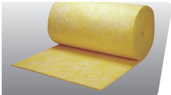
Spiral SG® is a fiberglass insulation designed for double-wall applications. The insulation comes in a variety of thicknesses to help optimize thermal and acoustical performance. It is made from rotary-process glass fibers bonded with a thermosetting resin, improving tensile strength and flexibility, and making it resistant to damage during installation.
