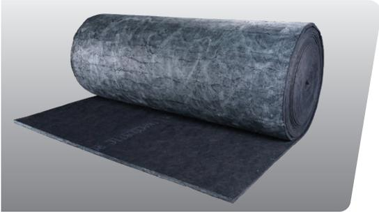
LinacouSTIC® RC-IG insulation is a premium, flexible, fiberglass duct liner made from strong glass fibers bonded with a thermosetting resin. The airstream surface is protected with JM's exclusive Reinforced Coating System, which combines our state-of-the-art Permacote® acrylic coating with a flexible glass mat reinforcement to provide a smooth air stream surface. On the opposite side of the airstream surface, LinacouSTIC RC-IG contains InsulGrip® a non-toxic, water-reactivated adhesive layer.
