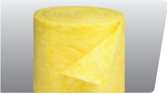
Microlite® Standard Duct Wrap is a lightweight, highly resilient, blanket-type, thermal and acoustical insulation made from flame-attenuated glass fibers bonded with a thermosetting phenolic resin.
