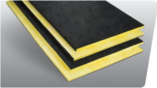
Linacoustic® R-300 is a rigid fiberglass board designed to line ducts in plenum spaces. The insulation has an airstream surface treated with the antimicrobial Permacote coating.
