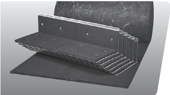
Linacoustic® RC-HP insulation is a flexible, fiberglass duct liner with higher density and enhanced acoustical control when compared to standard duct liners. The airstream surface is protected with JM's exclusive reinforced coating system, a glass mat surface coated with Permacote antimicrobial coating.
