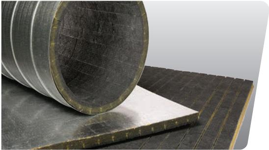
Spiracoustic Plus® is a fiberglass insulation designed to line spiral ducts. It has factory-made, evenly spaced kerfs to allow the material to easily conform to the inside diameter of spiral air ducts. The airstream surface and transverse edges are protected with JM's factory-applied Permacote coating. Spiracoustic Plus can save time and reduce weight when compared to some double-wall systems.
