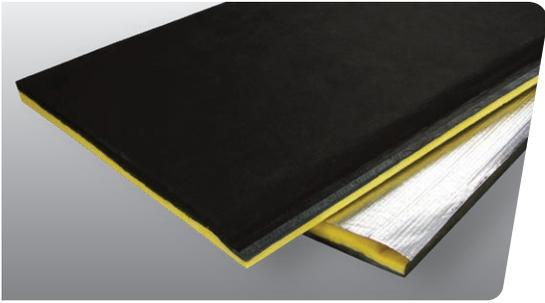
SuperDuct® RC is an FSK-faced fiberglass duct board insulation designed to be fabricated into rectangular ducts. Each board comes with a male or female shiplap to help make the fabrication process more efficient and accurate. The insulation itself has a glass mat airstream surface that is coated with the antimicrobial Permamate coating to improve durability and offer resistance to microbial growth.
