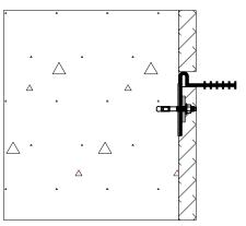
11) If expansion joint install expansion joint filler above and beneath waterstop embedment leg.
