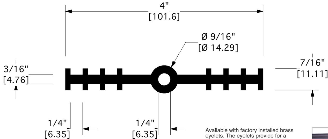
Available with factory installed brass eyelets. The eyelets provide for a convenient and durable tie-off point for wire tying the waterstop to the steel reinforcement prior to the concrete pour. JP Specialties installs the brass eyelets at 12" centers, between the last two ribs, to provide maximum resistance and rigidity to the poured concrete weight.
