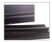
Available with factory installed brass eyelets. The eyelets provide for a convenient and durable tie-off point for wire tying the waterstop to the steel reinforcement prior to the concrete pour. JP Specialties installs the brass eyelets at 12" centers, between the last two ribs, to provide maximum resistance and rigidity to the poured concrete weight.
