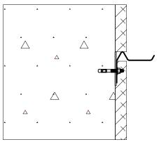
10) If expansion joint install expansion joint filler above and beneath waterstop embedment leg.
