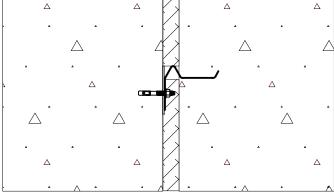
11) Allow installed retrofit waterstop system to cure for 24 hours before placing the second pour of concrete.
