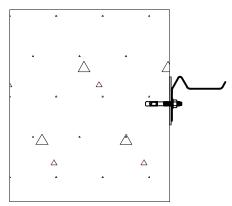
9) Hammer stainless steel wedge anchors into drilled holes, passing anchor through waterstop and epoxy gel bed. Repeat for all holes. Tighten anchor bolts.
