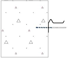
5) Using the stainless steel waterstop as a template, drill 1/4" holes 2-3/4" deep through waterstop and concrete. Clean out holes.
