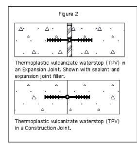
Due to aesthetics and functionality, concrete vaulting is usually the preferred method to contain hazardous chemicals. This is usually accomplished by placing the tank or process area on a concrete slab and surrounding it with short containment walls (usually 3 to 4 feet in height, [see figure 3]). Within the concrete joints (control, construction, and expansion), Earth Shield TPV Waterstop will span the joint preventing the passage of hazardous waste to the environment
