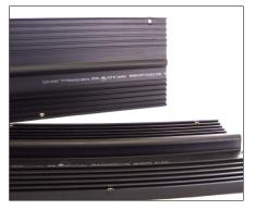
Available with factory installed brass eyelets. The eyelets provide for a convenient and durable tie-off point for wire tying the waterstop to the steel reinforcement prior to the concrete pour. JP Specialties installs the brass eyelets at 12" centers, between the last two ribs, to provide maximum resistance and disidity to the control of the concrete pour. rigidity to the poured concrete weight.
