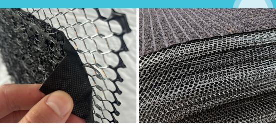
LathNet is a metal lath and drainage plane system that provides a continuous drainage plane between the lath and weather resistant barrier. The Masonry Advisory Council recommends that in exterior adhered masonry wall systems, a drainage mat be installed to drain any water that has penetrated to the flashing. A galvanized expanded metal lath, or diamond mesh, should be attached atop the drainage mat.
