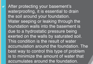
✓ Driwall™ Protection Board does this by eliminating hydrostatic pressure. Its open structure provides room for ample drainage, while a non-woven fabric separates soil from the water, allowing the water to move away from the foundation through the drainage pipe.
