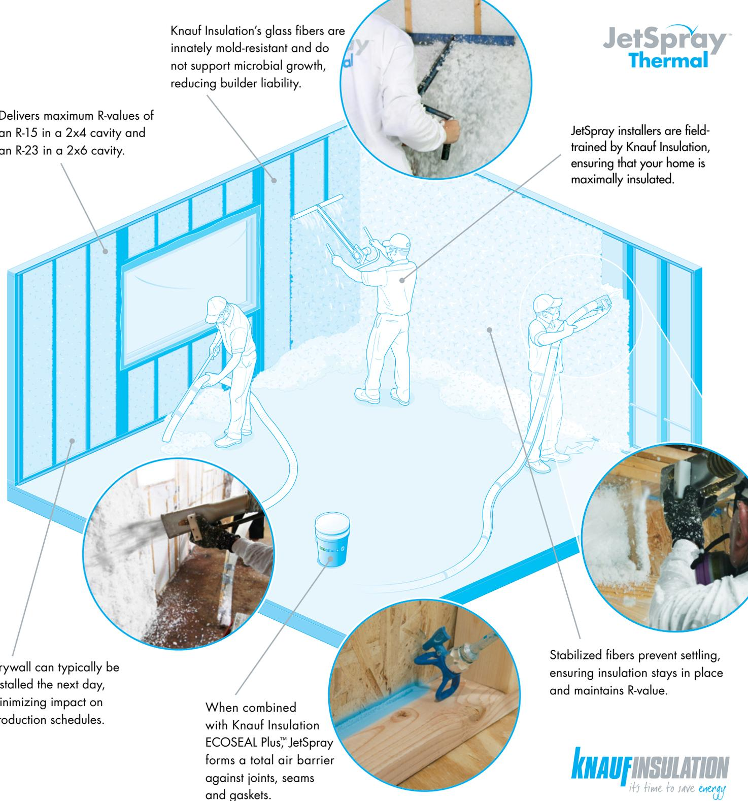
Drywall can typically be installed the next day, minimizing impact on production schedules.
