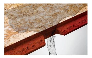
The RainChannel® self-draining notch system allows water to drain quickly from the surface. Combined with a moisture-resistant edge seal the RainChannel system helps fight moisture absorption and edge swell, reducing the need for sanding.
