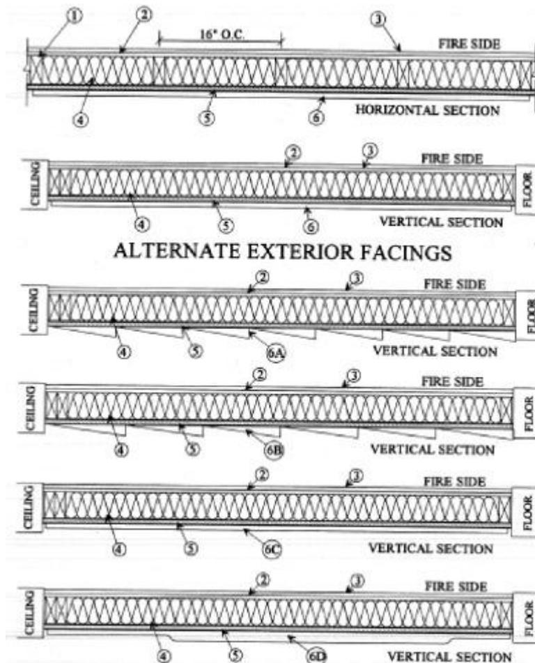
1. **Wood Studs** — Nom 2 by 4 in., spaced 16 in. OC in with two 2 by 4 top and one 2 by 4 bottom plates. As an option, nom 2 by 6 in., spaced 24 in. OC with two 2 by 6 top and one 2 by 6 bottom plates may be used in lieu of 2 by 4 studs and plates. Studs effectively fire stopped.
