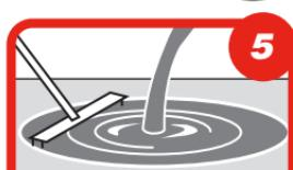
Ceramic tile and natural stone can be installed 3 hours after application. Floor coverings can typically be installed 16 to 24 hours after application.
