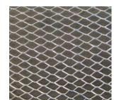
USE: Uses same mesh configuration as Diamond Mesh Lath but made with 1/4" dimple indentations spaced 1·1/2" o.c. each way. Used as exterior stucco base, column fireproofing and re-plastering over old surfaces. Available in galvanized only Paper conforms to Federal Specification UU-B-790A, type 1, grade D, style 2.
