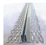
USE: To relieve the stresses of expansion and contraction in plaster or stucco. It is available in zinc or galvanized steel. Zinc should be used for exterior applications.
