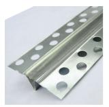
USE: To relieve the stresses from expansion and contraction across the joint in large ceiling and wall areas in drywall and veneer finish systems. It is used from floor to ceiling in long partition runs and from door header to ceiling. It is also recommended for repair of existing plastered masonry. Made of roll-formed zinc to resist corrosion, it has 3/32" grounds. Plastic tape protects 1/4" wide x 7/16" deep opening, and is to be removed after installation.
