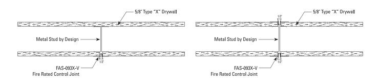
UL Systems available allowing installation on both or one-side of wall assembly. Consult UL System for details.
