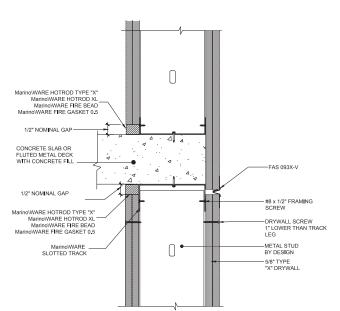
\*NOTE: SINGLE LAYER OF 5/8" TYPE "X" DRYWALL FOR 1 HOUR FIRE RATING, 2 LAYERS FOR 2 HOUR
