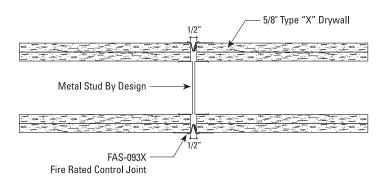
\*NOTE: SINGLE LAYER OF 5/8" TYPE "X" DRYWALL FOR 1 HOUR FIRE RATING, 2 LAYERS FOR 2 HOUR
