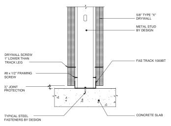
\*NOTE: SINGLE LAYER OF 5/8" TYPE "X" DRYWALL FOR 1 HOUR FIRE RATING, 2 LAYERS FOR 2 HOUR
