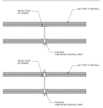
\*NOTE: SINGLE LAYER OF 5/8" TYPE "X" DRYWALL FOR 1 HOUR FIRE RATING, 2 LAYERS FOR 2 HOUR
