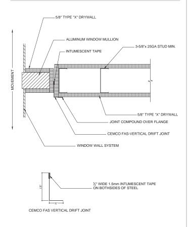
\*NOTE: SINGLE LAYER OF 5/8" TYPE "X" DRYWALL FOR 1 HOUR FIRE RATING, 2 LAYERS FOR 2 HOUR
