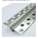
**USE**: To relieve the stresses from expansion and contraction across the joint in large ceiling and wall areas in drywall and veneer finish systems. It is used from floor to ceiling in long partition runs and from door header to ceiling. It is also recommended for repair of existing plastered masonry. Made of roll-formed zinc to resist corrosion, it has 3/32" grounds. Plastic tape protects 1/4" wide x 7/16" deep opening, and is to be removed after installation.
