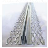
**USE**: To relieve the stresses of expansion and contraction in plaster or stucco. It is available in zinc or galvanized steel. Zinc should be used for exterior applications.
