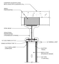
\*NOTE: SINGLE LAYER OF 5/8" TYPE "X" DRYWALL FOR 1 HOUR FIRE RATING, 2 LAYERS FOR 2 HOUR
