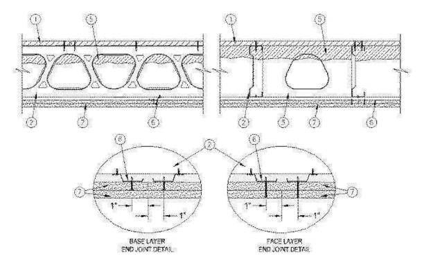
1. **Flooring** — Min 3/4 in. thick T & G plywood, min grade "Underlayment". Face grain of plywood to be perpendicular to joists with joints staggered. Plywood secured to joists with polyurethane based construction adhesive (optional) along with
