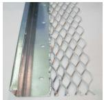
USE: As a plaster stop and as exposed trim around window and door openings. Can also be used at the junction or the intersection of plaster and other wall or ceiling finishes. Zinc should be used for exterior applications. Available with weep holes.
