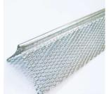
USE: Galvanized steel, used with one-coat or two-coat veneer systems to provide 3/32" grounds. With 1-1/4" fine mesh flanges, either stapled or nailed, provides an effective plaster key and eliminates shadowing
