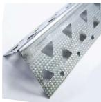
USE: A veneer bead used as an alternate to mini mesh veneer bead. It has a 1-1/2" leg and triangle cut-outs for one or two coat veneer plaster application. K-Rite corner bead is compatible with all brands of one and two coat plaster systems or multi-layer drywall construction. Perfect choice for repairs, column construction and new construction.
