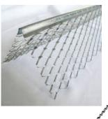
USE: Available in zinc or galvanized steel. Wide expanded flanges are easily flexed. Preferred for irregular corners. It provides increased reinforcement close to the nose of the bead. Zinc should be used for exterior applications.
