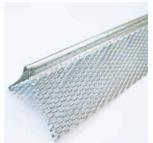
USE: Galvanized steel, used with one-coat or two-coat veneer systems to provide 3/32" grounds. With 1-1/4" fine mesh flanges, either stapled or nailed, provides an effective plaster key and eliminates shadowing
