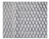
USE: For exterior stucco work over sheathing and as a plaster base over masonry walls. Self-furring embossed "V" groove holds the lath away from the surface to aid in the keying of stucco to the lath.
