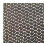
**USE:** Uses same mesh configuration as Diamond Mesh Lath but made with 1/4" dimple indentations spaced 1·1/2" o.c. each way. Used as exterior stucco base, column fireproofing and re-plastering over old surfaces. Available in galvanized only.Paper conforms to Federal Specification UU-B-790A, type 1, grade D, style 2.
