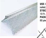
USE: Galvanized steel, used with one-coat or two-coat veneer systems to provide 3/32" grounds. With 1-1/4" fine mesh flanges, either stapled or nailed, provides an effective plaster key and eliminates shadowing
