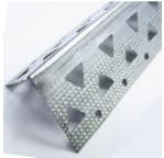
USE: A veneer bead used as an alternate to mini mesh veneer bead. It has a 1-1/2" leg and triangle cut-outs for one or two coat veneer plaster application. K-Rite corner bead is compatible with all brands of one and two coat plaster systems or multi-layer drywall construction. Perfect choice for repairs, column construction and new construction.
