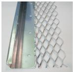
USE: As a plaster stop and as exposed trim around window and door openings. Can also be used at the junction or the intersection of plaster and other wall or ceiling finishes. Zinc should be used for exterior applications. Available with weep holes.
