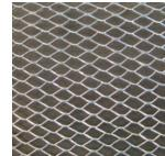
**USE:** Uses same mesh configuration as Diamond Mesh Lath but made with 1/4" dimple indentations spaced 1-1/2" o.c. each way. Used as exterior stucco base, column fireproofing and re-plastering over old surfaces. Available in galvanized only.Paper conforms to Federal Specification UU-B-790A, type 1, grade D, style 2.
