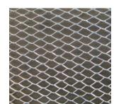
USE: Uses same mesh configuration as Diamond Mesh Lath but made with 1/4" dimple indentations spaced 1-1/2" o.c. each way. Used as exterior stucco base, column fireproofing and re-plastering over old surfaces. Available in galvanized only. Paper conforms to Federal Specification UU-B-790A, type 1, grade D, style 2.
