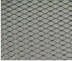
**USE:** Manufactured by slitting and stretching galvanized steel to form small openings to allow the keying of plaster so it will bond to the lath. Diamond Mesh Lath can be bent easily to create curved surfaces.
