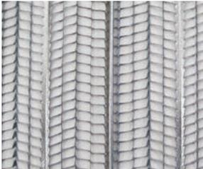
**USE:** Superior spanning characteristics over common expanded metal laths, suited for horizontal applications such as ceilings and soffits. Its 3/8" deep ribbed configuration is a self-furring feature. Designed for application on 24" on center.
