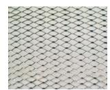
**USE:** Uses the same mesh configuration as Diamond Mesh Lath but made with 1/4" dimple indentations spaced 1·1/2" o.c. each way. Used as exterior stucco base, column fireproofing and re-plastering over old surfaces. Available in galvanized only. **SIZE:**
