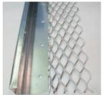
USE: As a plaster stop and as exposed trim around window and door openings. Can also be used at the junction or the intersection of plaster and other wall or ceiling finishes. Zinc should be used for exterior applications. Available with weep holes.
