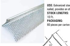
USE: Galvanized steel, used with one-coat or two-coat veneer systems to provide 3/32" grounds. With 1-1/4" fine mesh flanges, either stapled or nailed, provides an effective plaster key and eliminates shadowing
