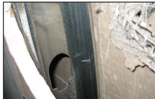
Soft body impact test using ViperStud.
