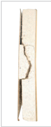
Rigid plastic wall panel - complete structural failure.
