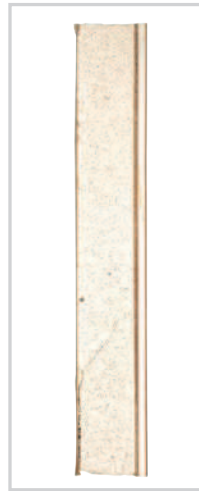
Induro™ FRP wall panel - nominal damage.
