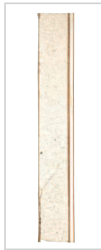
Induro™ FRP wall panel - nominal damage.
