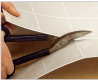
FRP panels can be easily cut with shears or a carbide tip saw.
