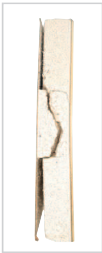
Rigid plastic wall panel - complete structural failure.
