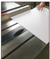
FRP Panels can be easily cut with a table saw.
