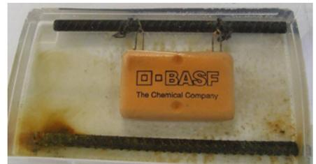
Figure 11 – MasterProtect Anode in Salt Water Solution
