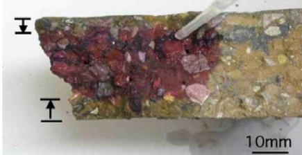
Figure 6 – Phenolphthalein Test of Carbonated Concrete (19)
