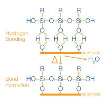
Figure 18 – Reaction of Alkylalkoxy Silane with Water (hydrolysis) to Produce Silanol and Alcohol Followed by Condensation and Bonding to the Pores of the Concrete Substrate (13)
