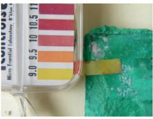
Figure 14 – pH of MasterProtect Anode Mortar After 6 Months (11)
