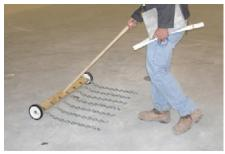
Figure 20 – Chain Pull Testing for Delaminations – ASTM D4580 Procedure B
