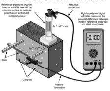
Figure 21 – Typical Half-Cell Testing Device (4)
