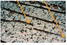
Figure 2 – Anodic and Cathodic Sites on Corroded Reinforcing Steel in Concrete in a Corrosion Cell in a Reinforced Concrete Structure
