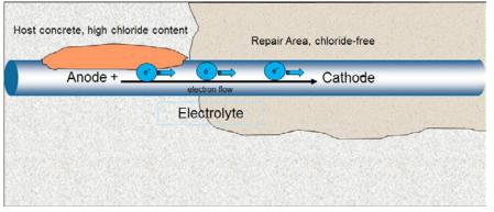
Figure 9 – Incipient Anode Effect at Concrete Patches
