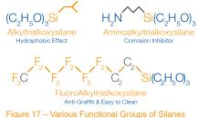
What is typically less understood is the functionality of silane molecules in the presence of an amine functional group. Depending on the chemical reaction that takes place, silanes can be created with different functionalities. MasterProtect 8000 Cl utilizes multiple silane functionalities to create different effects on the concrete substrate. These include the formation of a hydrophobic layer as well as a corrosion inhibition effect.
