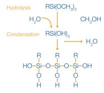
Aminoalkyltrialkoxysilanes can react within the concrete to disrupt the conductivity of the electrolyte. The reaction increases the resistivity of the concrete immediately adjacent to the reinforcing steel which in turn slows down the electrochemical reactions that make up the corrosion process. The reduction in the rate of the electrochemical reactions leads to a reduced corrosion rate which is known as corrosion inhibition.
