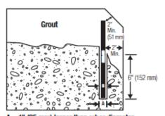
A = 1" (25 mm) larger than rebar diameter B = 1/2" (13 mm) diameter min. 3/4" (19 mm) recommended
