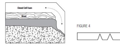
For shallow pours of 1–2 inches (25–51 mm), the wooden portion of the joint can be eliminated. Closed cell foam with notches to conform to vertical sides (see Figure 3) should be bonded directly to the concrete with or without a secondary seal.
