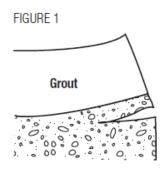
The potential for edgelifting is increased by these factors:
