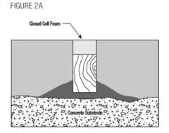
The wooden portion of the joint should be made from standard finished lumber that has a nominal thickness of 1 inch (25 mm). Actual thickness will be about ¾ (19 mm). Cedar is an excellent choice. It is resistant to water and oil, and is easily compressible.
