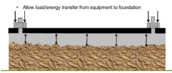
Grouting materials are selected based on the type of load they will support. *Dynamic loads* are associated with reciprocating equipment, motors, generators, turbines etc. *Static loads* are associated with columns or non-moving equipment.
