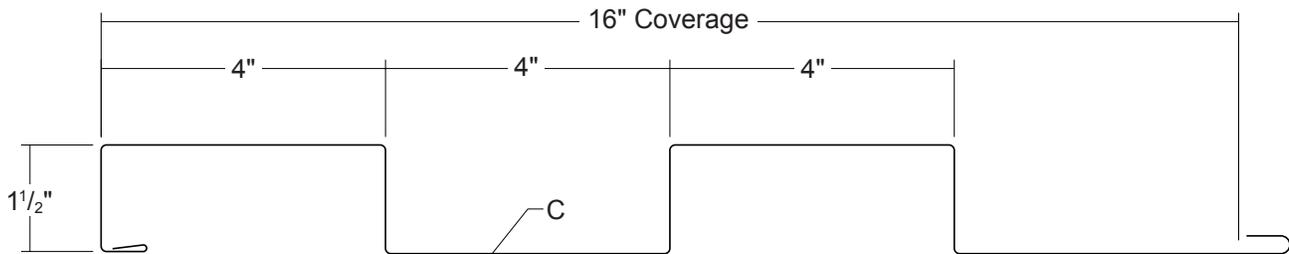
Panel can be produced in lengths from 6' to 30'.
