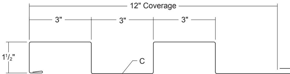
Panel can be produced in lengths from 6' to 30'.
