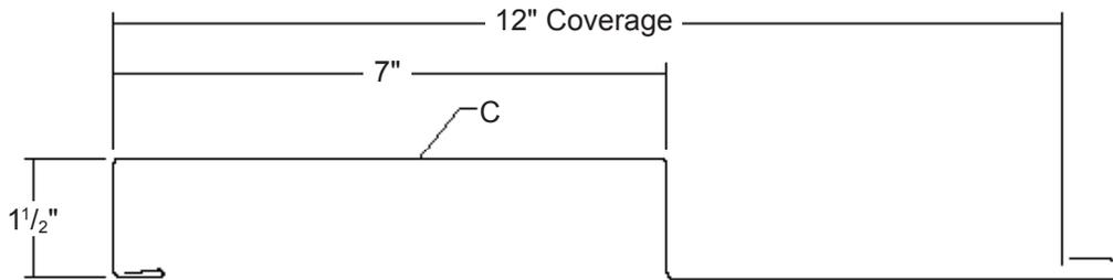
Panel can be produced in lengths from 6' to 30'.
