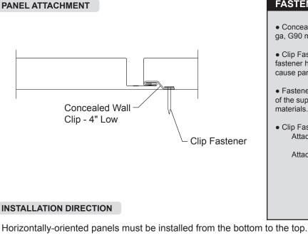
Vertically-oriented panels may be installed from the right-to-left or left-to-right.
