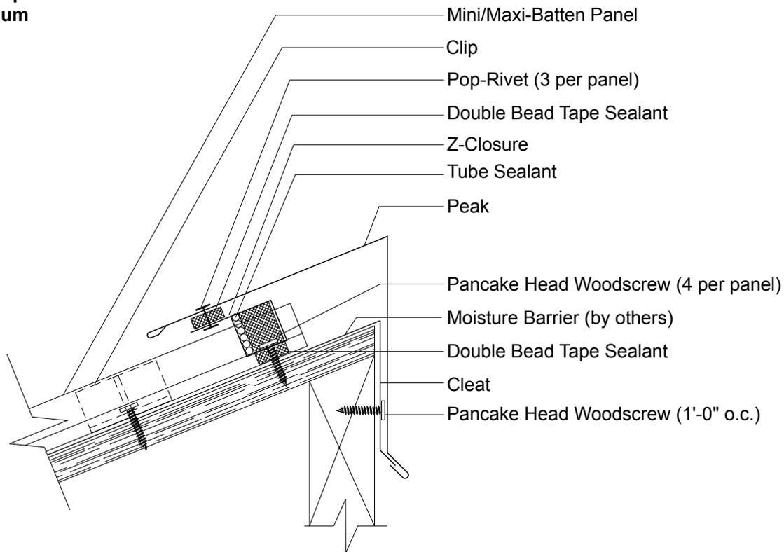
**Note: Z-Closures must be field cut and bent to fit between panel ribs (see Architectural Manual).**
