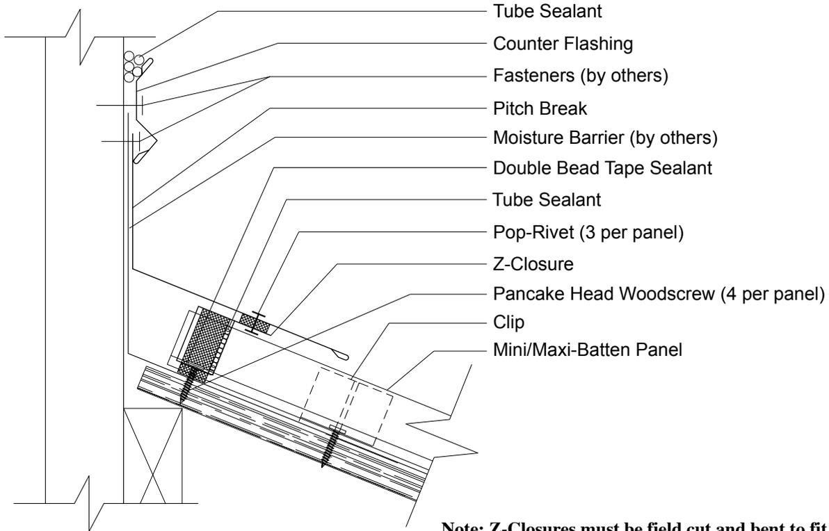
Note: Z-Closures must be field cut and bent to fit between panel ribs (see Architectural Manual).
