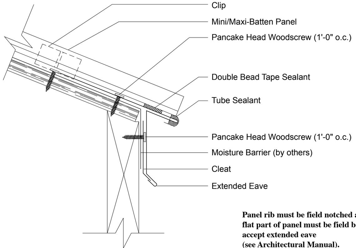
Panel rib must be field notched and flat part of panel must be field bent to accept extended eave (see Architectural Manual).
