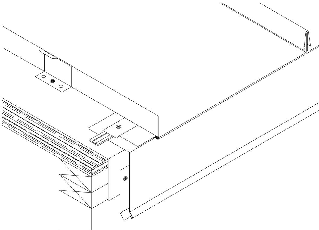
**Panel rib must be field notched and flat part of panel must be field bent to accept offset cleat (see Architectural Manual).**
