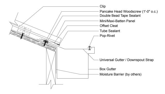
Panel rib must be field notched and flat part of panel must be field bent to accept offset cleat (see Architectural Manual).
