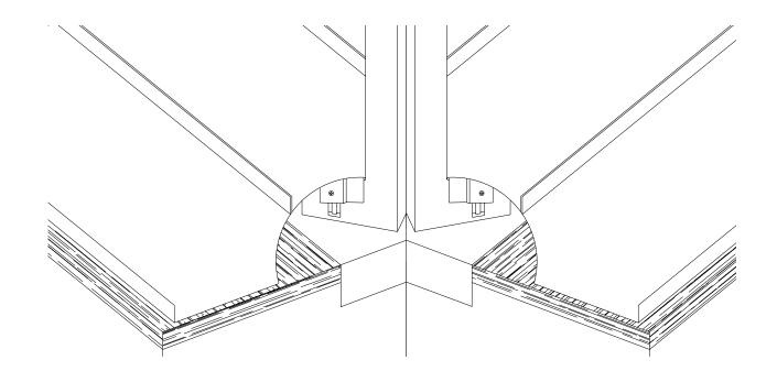
Panel rib must be field notched and flat part of panel must be field bent to accept offset cleat (see Architectural Manual).
