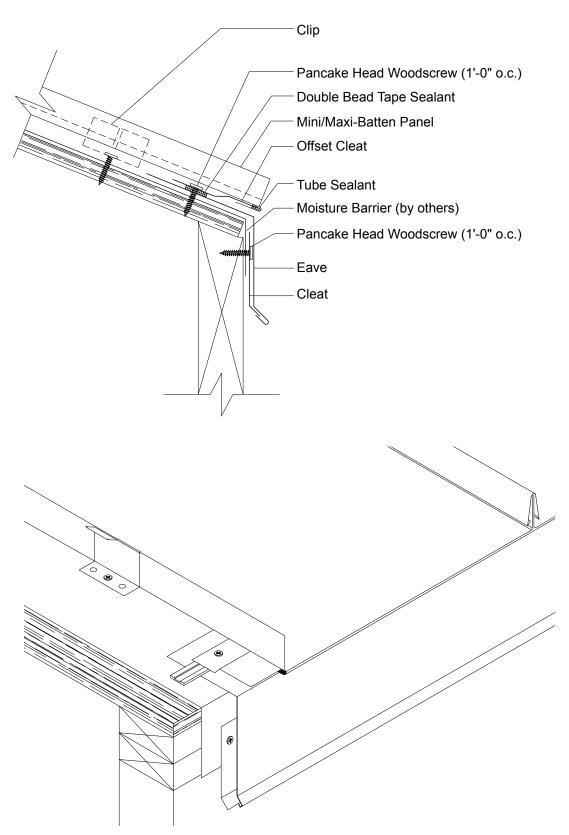
Panel rib must be field notched and flat part of panel must be field bent to accept offset cleat (see Architectural Manual).
