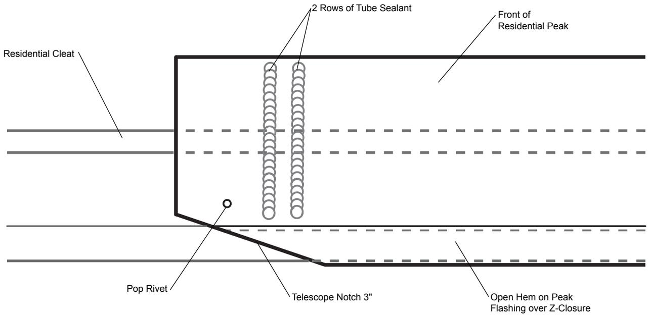
Peak Flashing Lap - Top View
