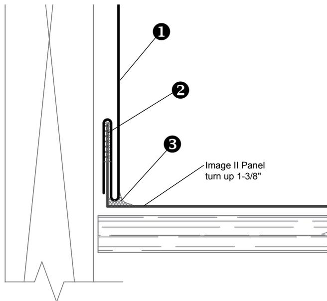
Residential Rakewall Flashing Lap Detail
