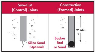
Example: In a typical 6" slab on grade, the control joints are cut 1 1/2" deep and the construction (cold) joints would be 6" deep. The filler would be installed 1 1/2" in control joints and 2" in thru-slab construction joints.
